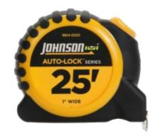
Auto-Lock<sup>™</sup> Features Self-Locking Blade, Push Button Retrieval, Blade-Gard<sup>™</sup> Nylon Coated Blade Resists Abrasion, Double Duty 2-Sided Printed Blade, Speed-Read Blade Features Fractional Graduations Every 1/8", Tiger Claw<sup>™</sup> 4 Rivet Blade Hook, Impact Resistant Ergonomic Co-Molded Rubberized Case, Models: 1804-0012 (12' x 5/8" blade width), 1804-0016 (16' x 1" blade with) and a 1804-0025 (25' x 1" blade width) tape measure
