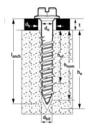
Slotted hex head version pictured, flat head length is measured from top of head to tip of anchor.
